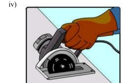
Use circular saw blade for cutting Marklon Polyglass® Polycarbonate Solid Sheet.
