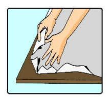
To install, 50mm of protective film should be peeled off from the edges of the sheet to allow clean sheet insertion into the glazing system.
