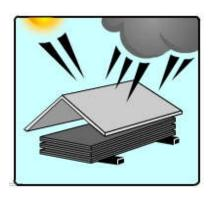
Sheets should be kept indoor, protected from sunlight and rain fall by an appropriate opaque waterproof roof cover.
