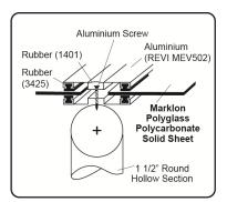
Make sure the support structure is clean and dry. Do not directly screw the sheet, only use aluminium clapping for joining. Must leave a gal of at least 5mm in between sheets for thermal expansion and contraction. A minimum slope of 5° roof pitch is recommended to allow adequate rain water run-off.
