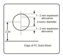
Use only new or sharp ground steel or carbide tipped drills. All holes must be drilled at least 40mm from the edge of the sheet. All holes must be at least 4mm bigger than screw for thermal expansion and contraction.
