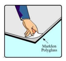
Marklon Polyglass® Polycarbonate Solid Sheet's is produced with a protective PE film on one or both sides which should be kept on until the panel is fastened. The UV protected side is to be faced towards the sun and is marked with printed film (Marklon Polyglass®)
